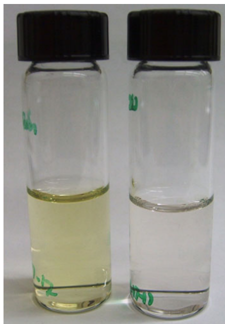
Fig. 1 Effect of 300 nm irradiation on 20 nm AgNP suspensions ( 4.0 \text{ mg L}^{-1} , commercial). Unexposed control suspension retained the characteristic yellow color (left) while exposed samples ( \approx 8,000 min) became near colorless (right). (Color figure online)
